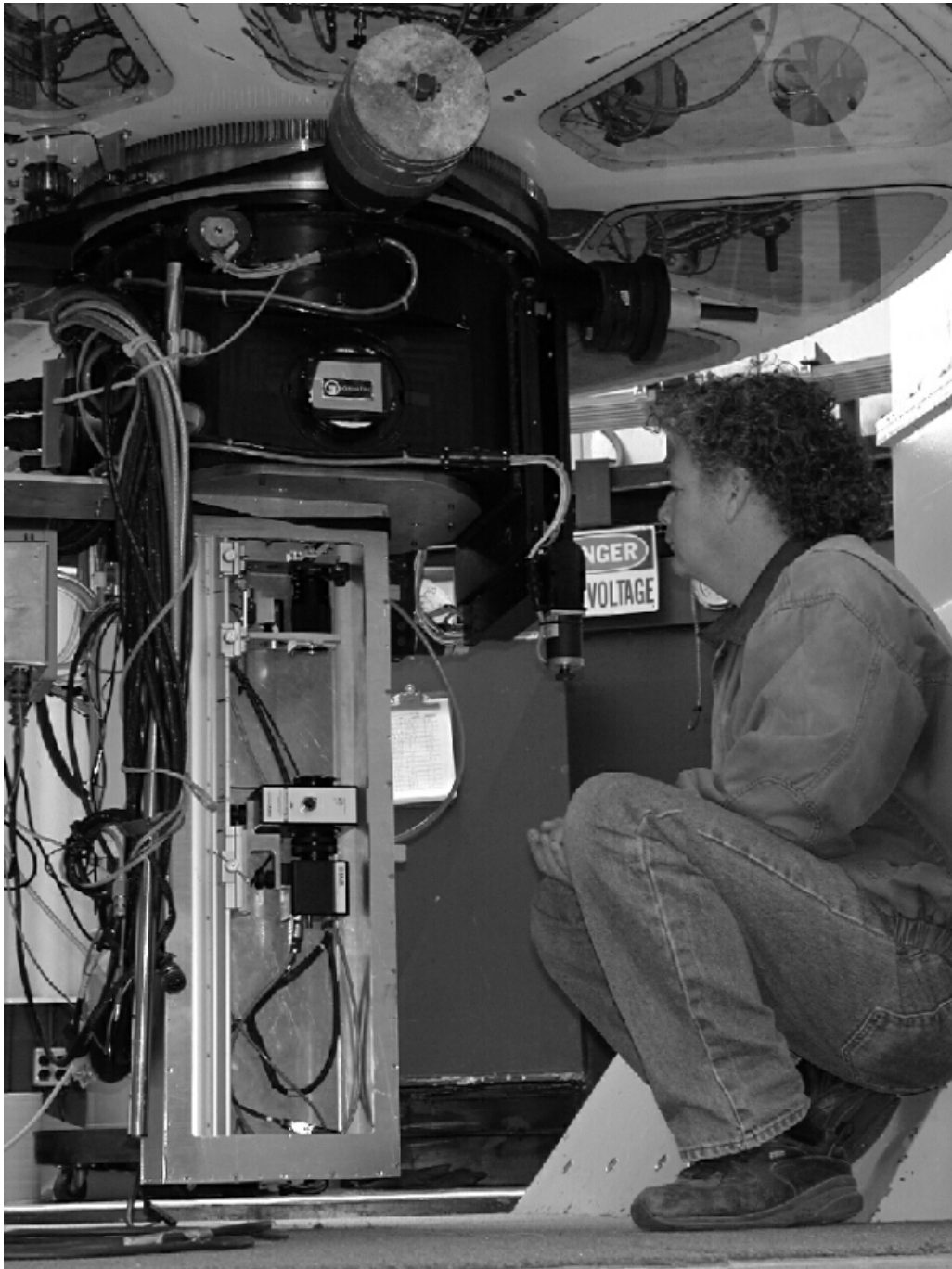
Figure (2) LBT SCIDAR instrument on the VATT 1.8meter telescope with the SCIDAR observer shown for scale. The detector position is set to -3.5 km or 157 mm behind the pupil plane.
